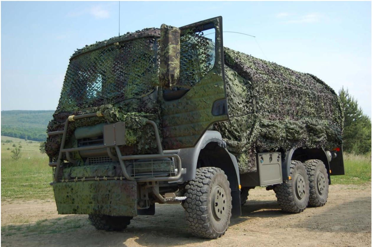
Fig.2. Full mobile camouflage on Tatra truck 810.
