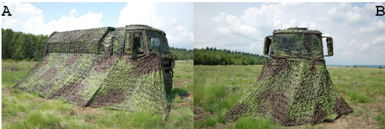
Fig.3. Combined camouflage on Tatra 810 consisting of mobile camouflage and additional nets. A) Right view of the vehicle B) Front view.
